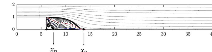
The reattachment point  $x_r$  is where the mean skin friction coefficient equals to zero:
