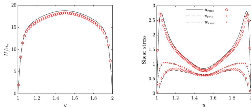
The iLES results are verified with DNS data. The comparison between the time- and spanwise-averaged of the streamwise velocity is in a good agreement.
